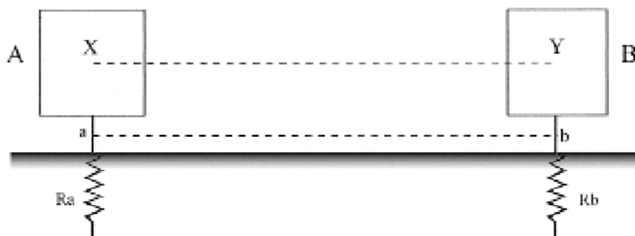
Figure 8-3 Earthing problems arising when equipment is interconnected
