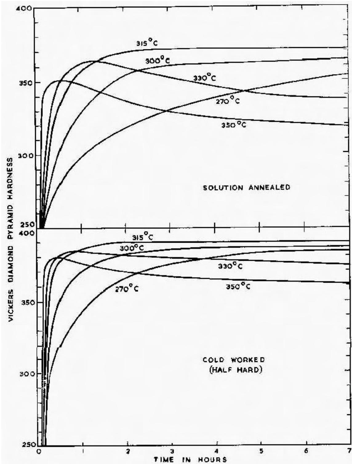
Figure 8 - Effect of precipitation heat treatment on the hardness of beryllium copper (Beryllium and Copper Alloys Ltd)
