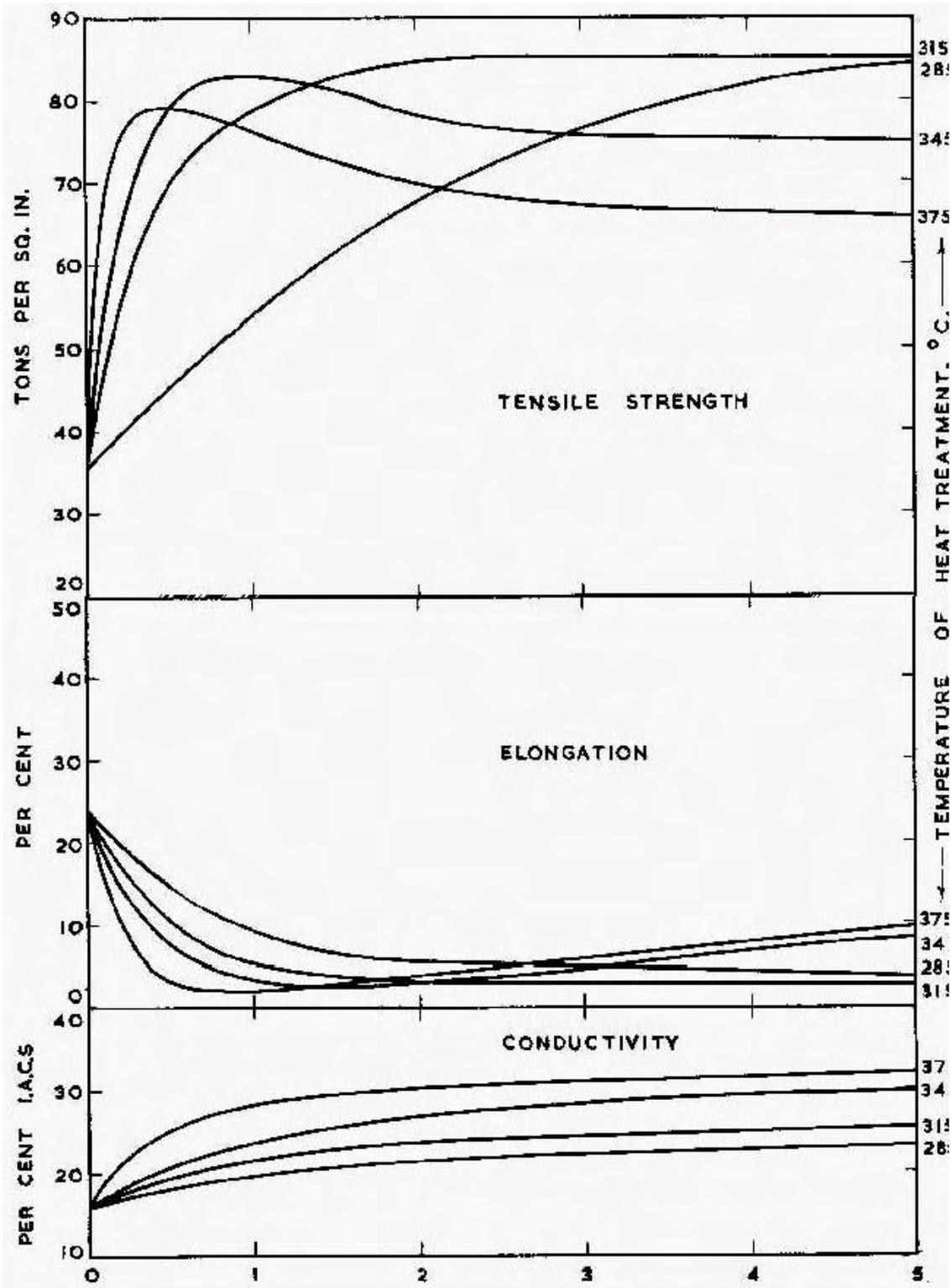
Figure 4 - Effect of precipitation heat treatment on quarter hard beryllium copper (Beryllium Corporation)
