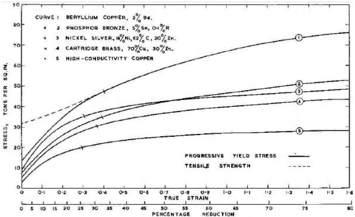
Figure 2 - Typical strain-hardening curves for copper, beryllium copper and several other copper alloys.
