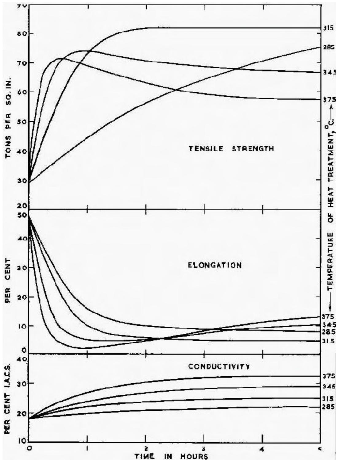
Figure 3 - Effect of precipitation heat treatment on solution-annealed beryllium copper (Beryllium Corporation)
