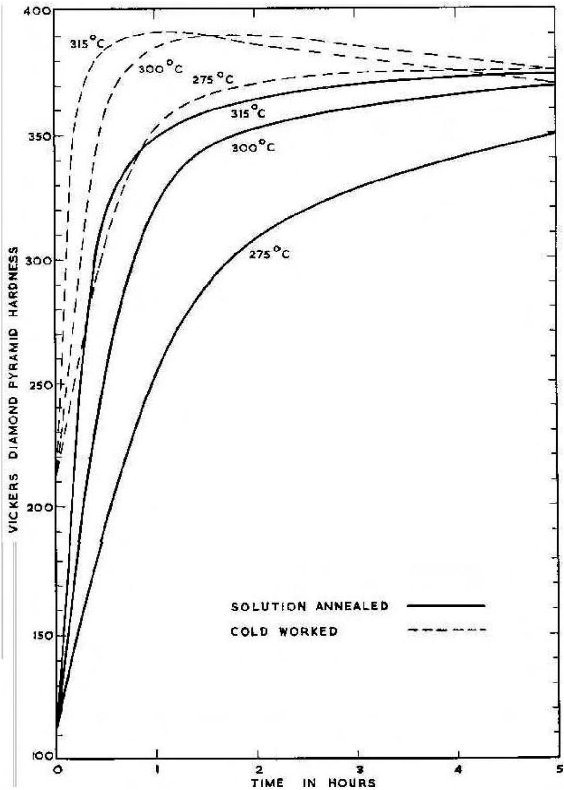
Figure 7 - Effect of precipitation heat treatment on the hardness of beryllium copper (Johnson, Matthey & Co Ltd)
