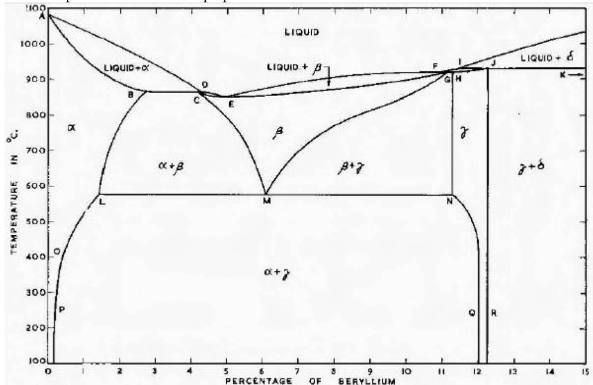
Figure 1 - Equilibrium diagram of the copper-beryllium system (copper-rich alloys)
