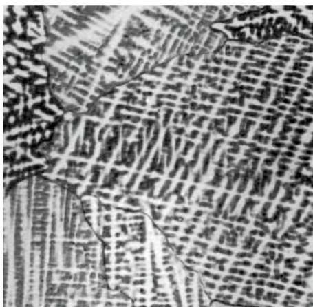
The microstructure shows coarse grains with a dendritic structure made visible by etching deeply with alcoholic ferric chloride. This reagent reveals the changes in composition due to coring.
