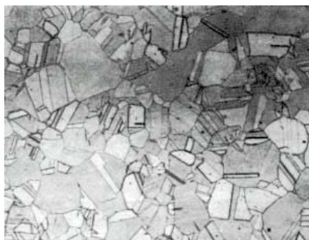
The microstructure shows twinned equiaxed  $\alpha$  grains. Uniform attack of the specimen during etching indicates that the structure is homogeneous. Coring in brass is much less persistent than in copper-tin and copper-nickel alloys.
