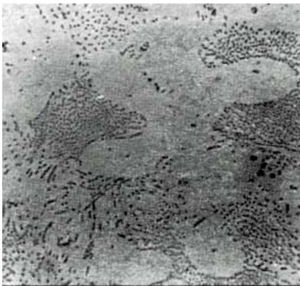
This microstructure shows areas of primary surrounded by the eutectic consisting of  $\alpha$  and blue chromium particles. The precipitate responsible for hardening is not visible at this magnification.
