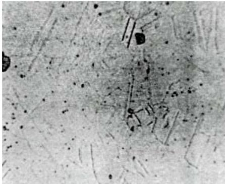
This specimen contains small spherical particles of  $\beta$  in the fine-grained  $\alpha$  matrix. Not all commercial alloys contain the  $\beta$  phase. It generally only occurs where there has been incomplete suppression of the transformation during cooling from elevated temperatures.
