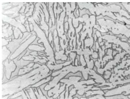
This specimen shows large  $\beta$  grains containing a Widmanstätten precipitate of  $\alpha$  which is etched slightly lighter in colour.
