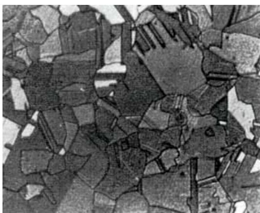
This microstructure shows twinned equiaxed grains and a complete absence of the Cu<sub>2</sub>O eutectic characteristic of tough pitch copper. Strong contrast between the grains is visible because of the use of alcoholic ferric chloride solution as etchant. This reagent is suitable for the metallographic preparation of most copper alloys, but attack is rapid and care is necessary to avoid over-etching and staining.
