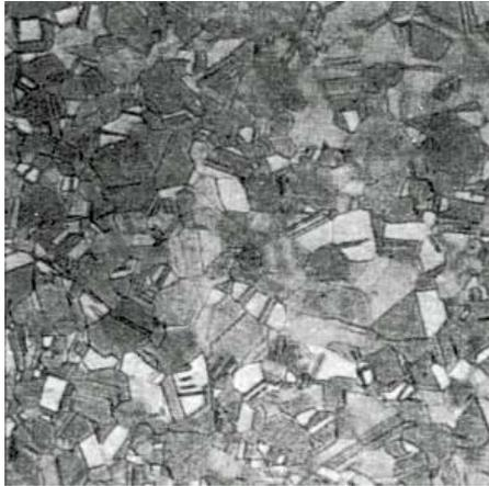
This specimen shows the typical recrystallised structure of twinned equiaxed grains.
