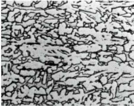
This specimen shows areas of  $\beta$  slightly elongated in the direction of working, in a matrix of  $\beta$ . The body-centred cubic  $\beta$  phase does not develop annealing twins. Twins are, however, present in the  $\alpha$  and would be revealed by deep etching. The lead (which has been added to improve machinability) appears as dark elongated particles.
