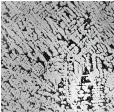
The microstructure shows copper dendrites interspersed with globules of lead which are darker in colour.
