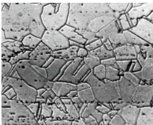
Hot working has broken down the cast structure to give twinned equiaxed grains. The Cu<sub>2</sub>O eutectic particles have been aligned in the direction of working and their distribution is no longer confined to grain boundaries. All traces of porosity have been removed. The grain structure is lightly delineated by the use of ammoniacal hydrogen peroxide etchant.
