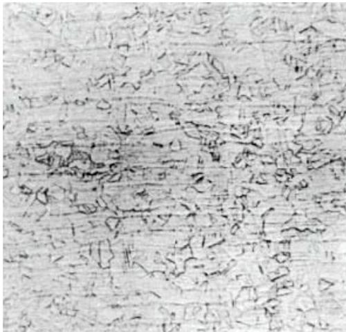
This alloy has a single-phase structure. Hot working has broken down the cast structure to give twinned equiaxed grains. Some banding is apparent which is the remains of the dendritic coring from the cast structure. The etchant used to prepare this specimen produces a minimum of structural relief and is recommended for the examination of all copper nickel alloys.
