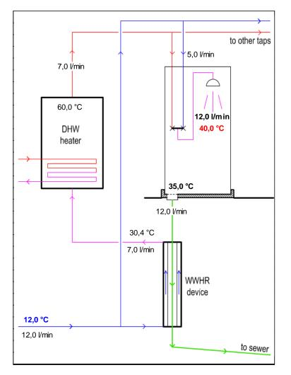
Domestic hot water needs = 23,4 kW (40°C-12°C) x 12 l/min x 60 min/h x 1,16 Wh/°C l
