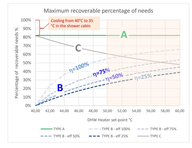
The **recoverable** part of needs strongly depends on connection type A - B - Cbut also on dhw heater set-point (operational choice)
