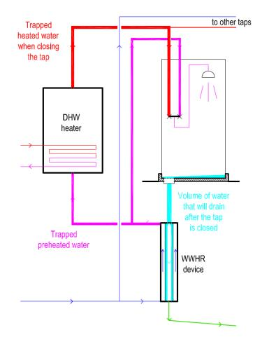
When closing the shower tap, the heat trapped in the system that has been accounted as recovered heat will not be actually recovered. This includes heat:
