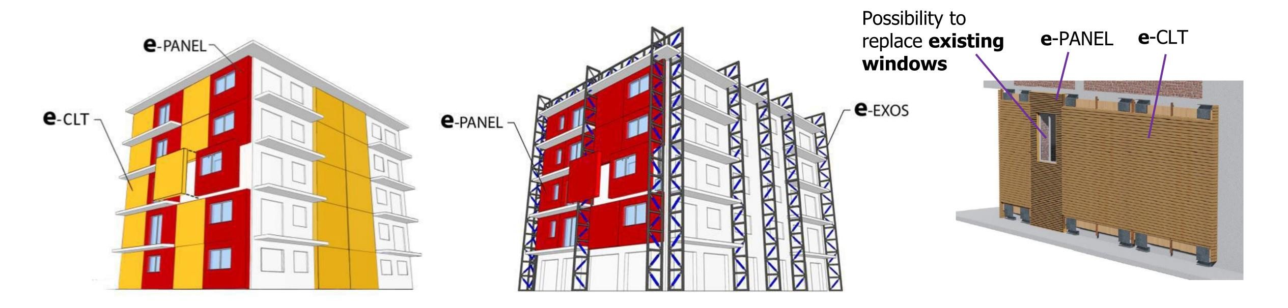
e-PANEL: prefabricated plug-and-play modules with timber-framed structure and bio-based insulation
