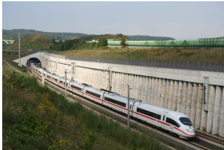
Figure 6 – A German ICE high-speed train, consisting of two units of 8 MW each (photo by S. Terfloth, licensed under Creative Commons ( cc-by-sa/2.0 )).
