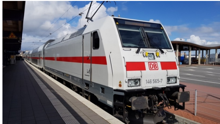
Figure 5 – Deutsche Bahn Class 146 Electric locomotive (Photo by Clic, licensed under Creative Commons ( cc-by-sa/4.0 )).
