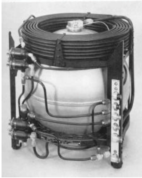
Aircraft liquid oxygen converter – 30 litre capacity. The container comprises two spheres, one within the other, with the space between evacuated to a vacuum. Because of its low thermal conductivity nickel silver tubing is used to connect the two chambers.
