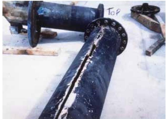
Figure 10 - Corrosion of nickel aluminium bronze pipe along seam weld due to residual beta-phase
