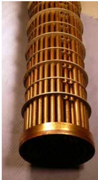
*Figure 2 - 90/10 copper-nickel tubing in an oil cooler*
