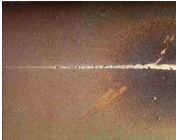
Figure 8 - Erosion corrosion of a scratch on an aluminium brass condenser tube due to excessive chlorination
