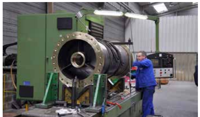
Figure 17 - Column pipe (Courtesy Inoxyda SA, France)
