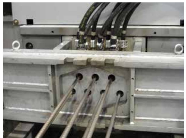
Figure 70 - Horizontal 7 strand bar casting (Courtesy Alfred Wertli, Switzerland)
