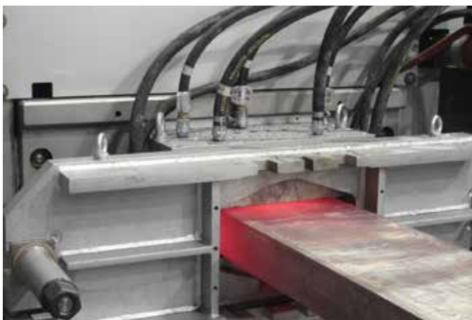
Figure 69 - Horizontal slab casting (Courtesy Alfred Wertli, Switzerland)
