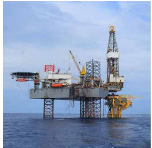
Figure 20 – Jack-up rig units which use additional bearings and bushings in the cranes and mooring winches as well as the jack-up gearboxes
