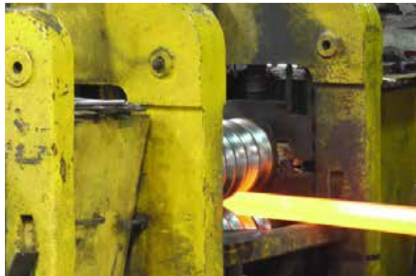
Figure 75 – Hot rolling (Courtesy Pro-Roll Ltd, Sheffield, UK)
