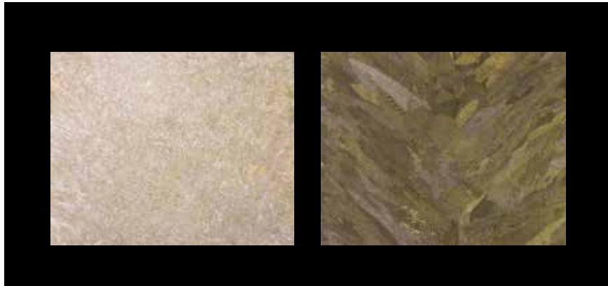
Figure 71 – Grain refining in continuous casting (Courtesy Copper Alloys Ltd, Stoke on Trent, UK)
