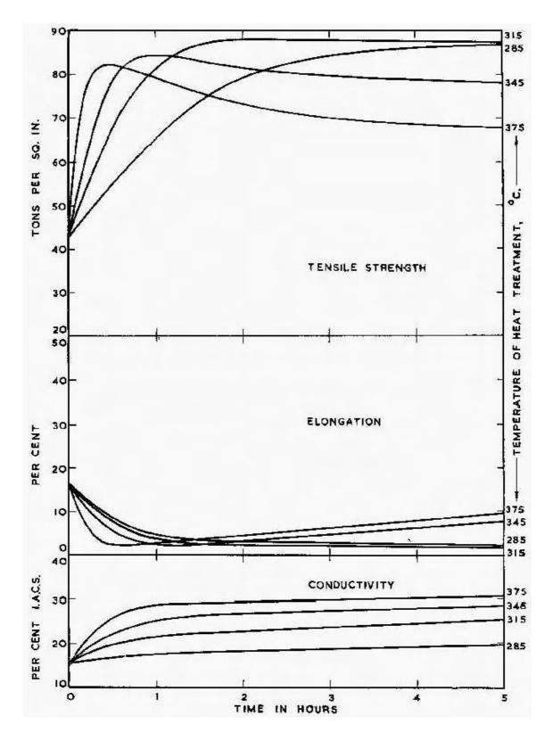
Figure 5 - Effect of precipitation heat treatment on half hard beryllium copper (Beryllium Corporation)
