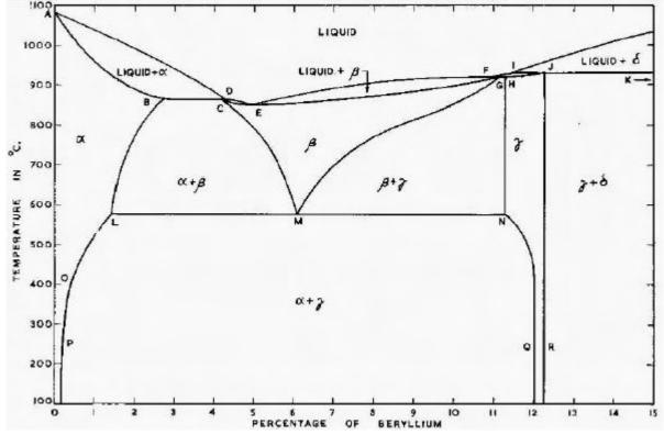
Figure 1 - Equilibrium diagram of the copper-beryllium system (copper-rich alloys)
