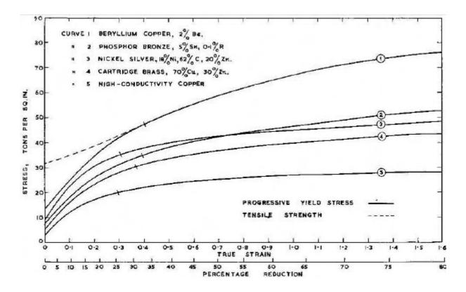
Figure 2 - Typical strain-hardening curves for copper, beryllium copper and several other copper alloys.
