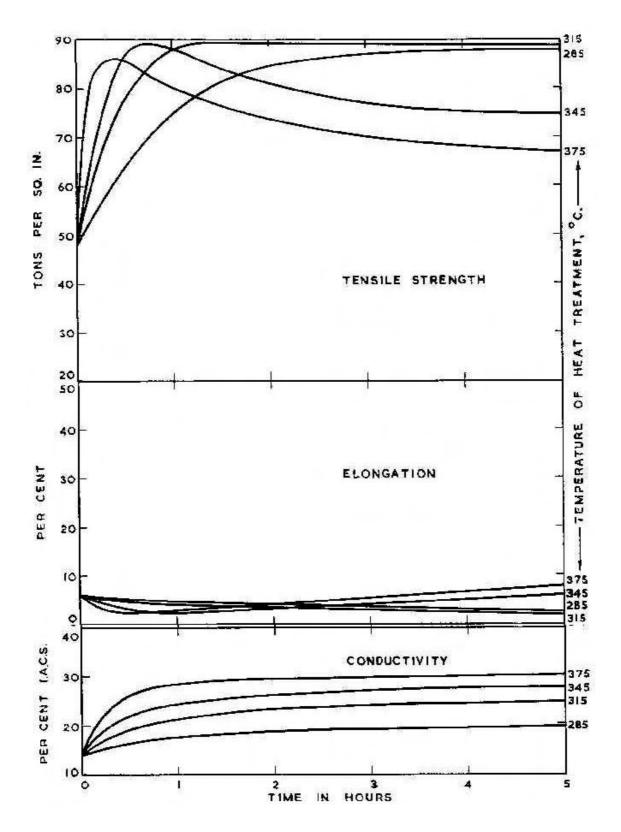
Figure 6 - Effect of precipitation heat treatment on hard-worked beryllium copper (Beryllium Corporation)
