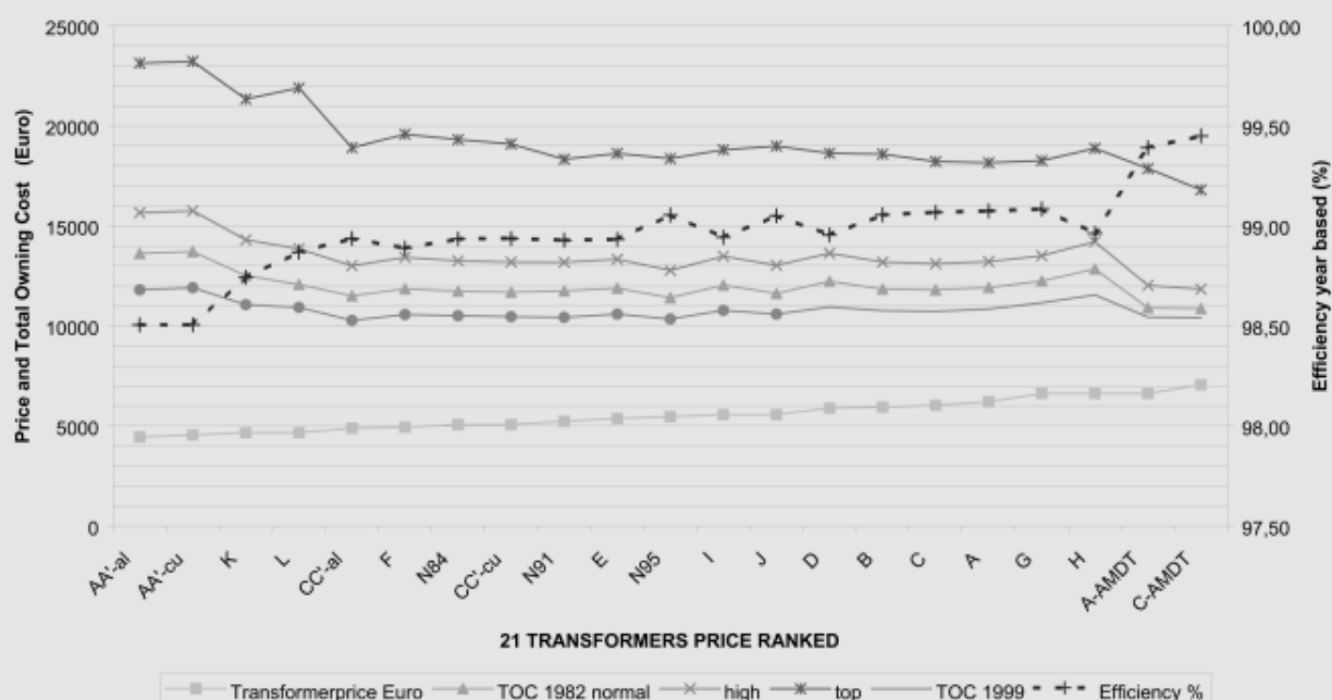
Transformers 400 kVA Evaluated Project Groningen (NL) 1982-1999 at peak load / rated load = 0,6
